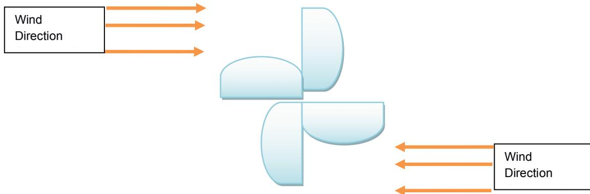
**Figure 2.1.1:** Illustration of a wind turbine working principle
