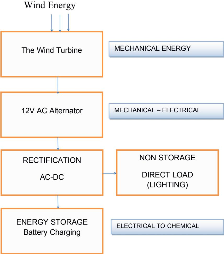
**Figure 1.5:** Block Diagram of Wind Energy conversion into electrical energy.
