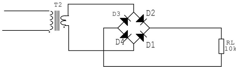
**Figure 2.1.4:** Circuit of a bridge rectifier
