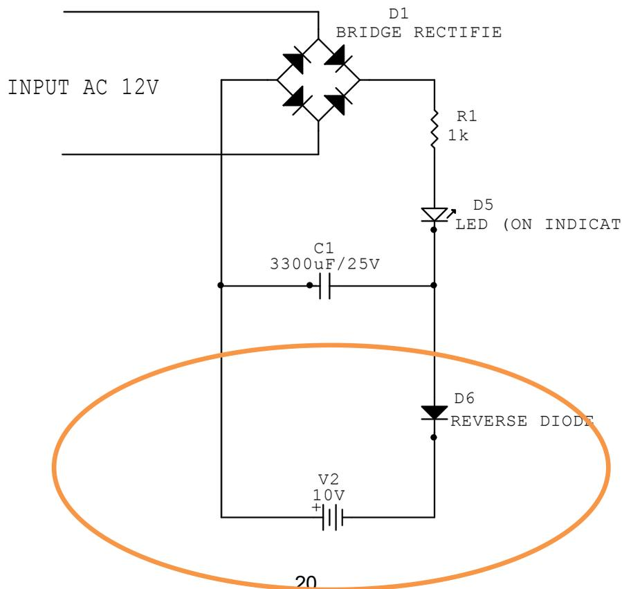
**Figure 2.1.5:** The battery charging
