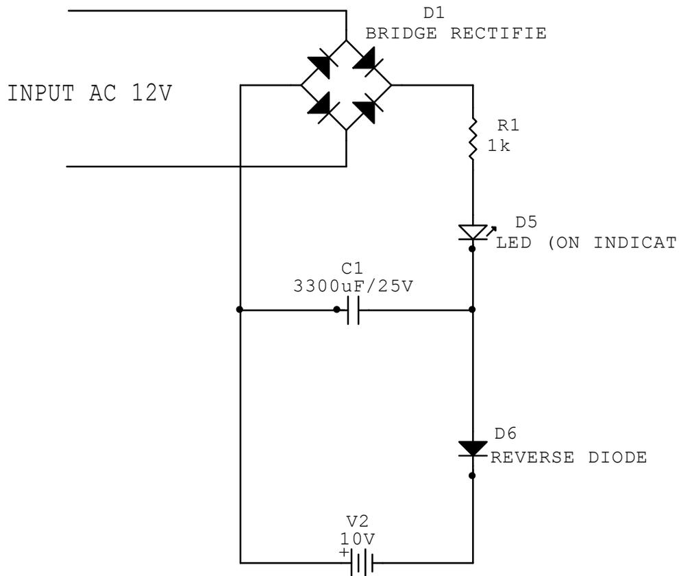
**Figure 2.1.3** Rectification Circuit
